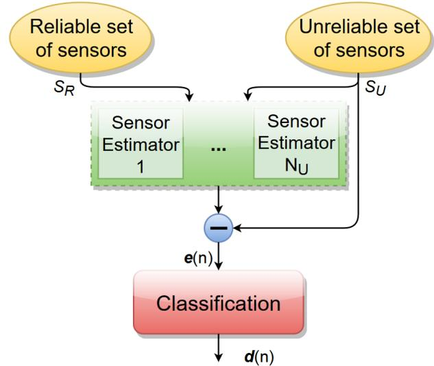
Fig. 1: The proposed system architecture for SFDIA.
